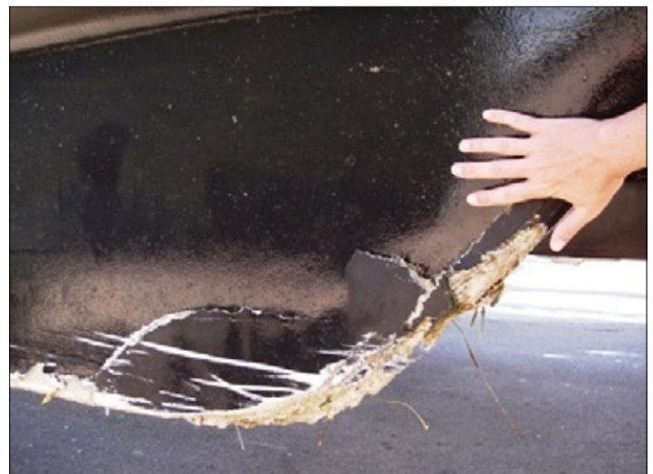
The extent of the damage - shattered fiberglass on the hollow starboard keel
